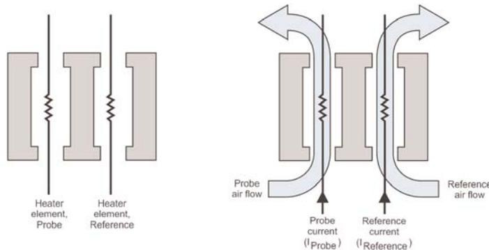
**LEFT:** Dual analysis is achieved with heater elements positioned in separate flow chambers.
