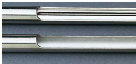
Top: electropolished finish, surface roughness average number: 5-10. Bottom: conventional finish, surface roughness average number: 23-27.
