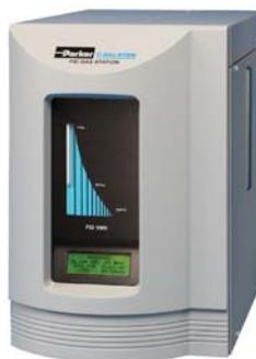
Parker Balston's FID-1000 Gas Station provides both UHP grade hydrogen fuel gas and zero grade air (<0.1ppm THC) for flame ionization detectors on gas chromatographs. The system is specifically designed to supply fuel gas to either 1 or 2 FIDs and to support flame thermionic and flame photometric detectors.
