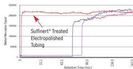
treated electropolished tubing did not adsorb methyl mercaptan to any measurable extent, delivering a representative sample with no delay. The untreated electropolished tubing, in contrast, totally adsorbed methyl mercaptan for more than 75 minutes, and the sulfur gas level did not stabilize until approximately 130 minutes. Conventional 316L seamless tubing totally adsorbed methyl mercaptan for more than 90 minutes, and the sulfur gas level did not stabilize until approximately 140 minutes.
