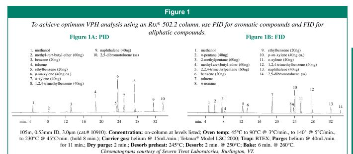
The PID is used to identify target VPH analytes, defined as benzene, toluene, ethylbenzene, *m*-xylene, *p*-xylene, *o*-xylene, naphthalene, and methyl-*tert*-butyl-ether. The VPH method identifies all of the aromatic compounds after *o*-xylene to naphthalene. The reason for the distinction of aromatic from aliphatic compounds rests on current data, which suggests aromatic compounds are more toxic.
