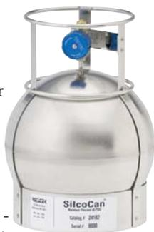
For ultimate inertness, we treat SilcoCan™ air monitoring canisters with our unique Siltek® passivation technology. Even highly active components, at low parts-per-billion concentrations, can be stored without loss. The valve is a high quality, metal-to-metal seal, 2/3-turn valve with metal diaphragms. Both stainless steel and Siltek®-treated valves are available, in both the 2-port and 3-port configurations.
