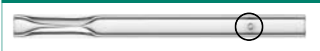
Figure 1—The drilled hole in a Uniliner® injection port liner makes direct injection possible with EPC systems by equalizing pressure in the injection port.
