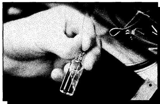
Figure 2 - Confirm column flow by submerging the column outlet in a vial of methanol.
