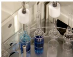
Alcohols, crude oils, and alkanes such as hexane can be sealed at ambient temperatures with purge gas injection. Injecting an inert purge gas (i.e. argon or nitrogen) into the ampule after filling displaces both oxygen and solvent vapor from the ampule, reducing vapor pressure and flammability.
