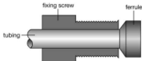
*These mounting instructions are for tubing with 1.6 and 3.2 mm outer diameter.*
