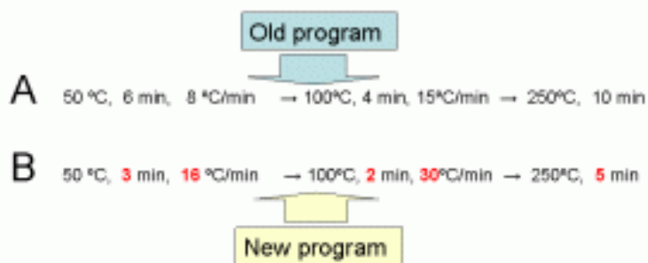
Fig.8 Example of calculation for a 30m column moving from 30 to 60 cm/s
