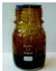
loading achieve is 50% weight/weight and shows how samples containing solids can be loaded, without affecting operation or performance of the HPLCCC instrument.
