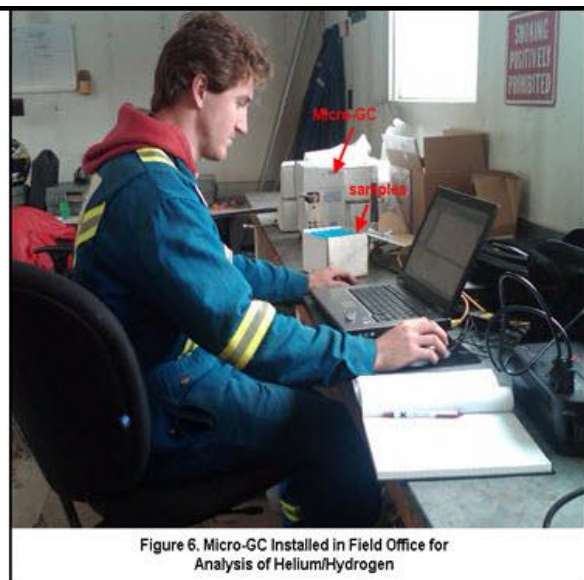
Figure 3. Analysis of Hydrocarbons and CO 2 by Gas Chromatograph and Helium/Hydrogen by Micro-GC in Field Hut
