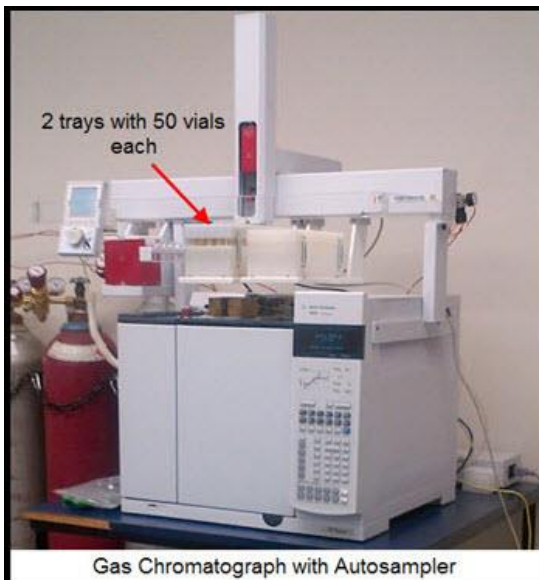
Figure 3. Analysis of Hydrocarbons and CO 2 by Gas Chromatograph and Helium/Hydrogen by Micro-GC in Field Hut
