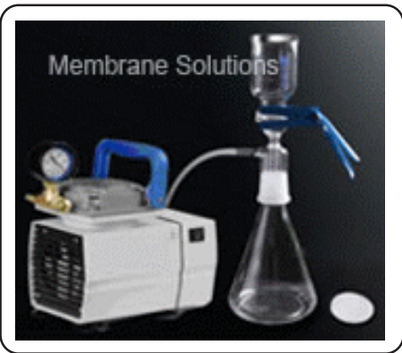
Solvent Filtration System
