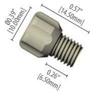
002244 PEEK™ nut for 1/8" OD tubing 1/4•28, natural
