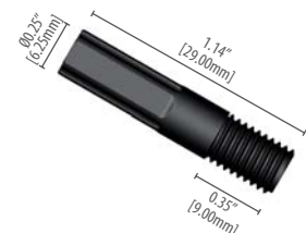
008NF32-YL5B Long nut for 1/8" OD tubing, 1/4•28, black
