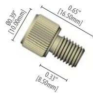
002222 PEEK™ nut for 1/8" OD tubing, 1/4•28
