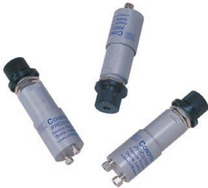
The Vici combo regulator is a combination regulator and shut-off valve. The pressure is set using the screwdriver adjustment in the center of the on/off knob. Turning the knob counterclockwise provides positive shutoff, while clockwise rotation restores gas pressure to within 0.05 psi of the setpoint.
