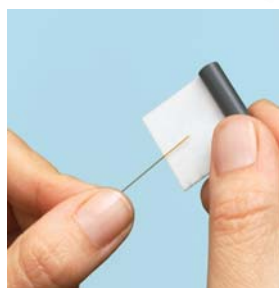
Check the cut against the white of the scoring wafer. Look for a clean, square cut.
