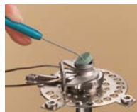
Remove septum without damaging an expensive weldment.
