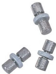
The 1/32" external union is specially designed for use with capillary columns in GC. It has very low mass and does not require wrenches to seal. Use only with one-piece fused silica adapters, since metal ferrules will distort the detail. Order fused silica adapters separately (*see box at left*).
