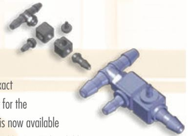
The Build-a-Part system is based on combining interchangeable components, joining junction blocks and luer, hose barb or threaded features to create the desired configuration. The features are bonded to the junction blocks using commonly available adhesives. Junction blocks and features may be bonded together to create multi-port, multi-axis products that receive and redirect fluid flow in whatever direction the designer desires. The only limitation is the designer's imagination.
