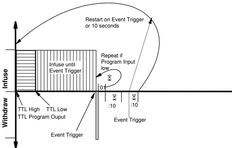
This example demonstrates a complex interaction with external equipment, such as synchronizing with another syringe pump. The Program includes a variety of interactions with external equipment, which demonstrates the various control possibilities of the NE-4000.
