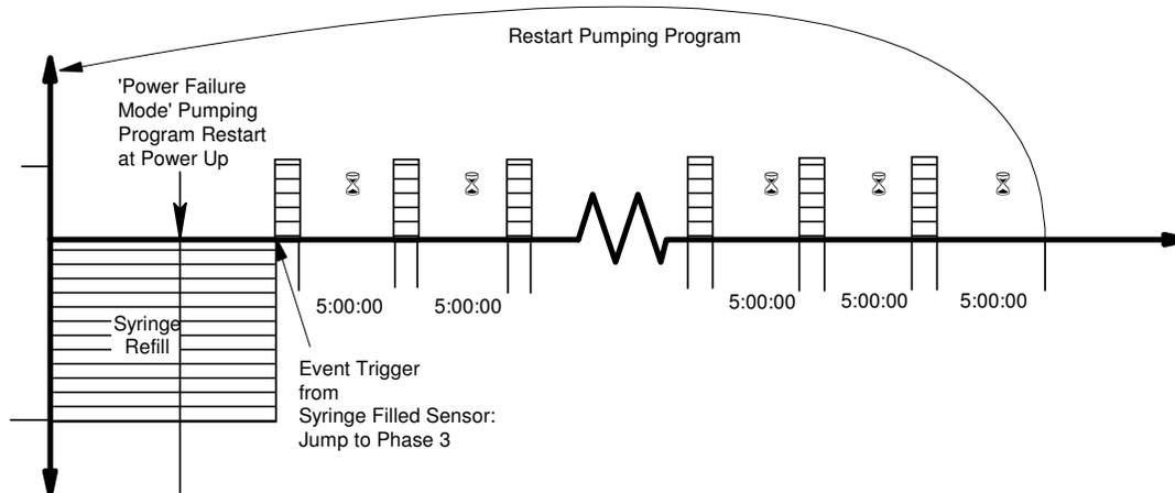
The following is an automated dispensing Program for a NE-4000 syringe pump equipped with a 'Syringe Filled Sensor' attached to the TTL I/O connector, and a valve system to refill the syringe from a reservoir. It is also assumed that the 'Power Failure' mode is enabled.
