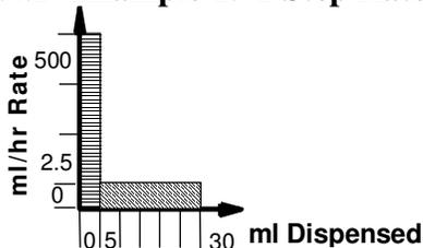
Infuse 5.0 mL at 500 mL/hr, and then infuse 25.0 mL at 2.5 mL/hr. Then stop the pump.
