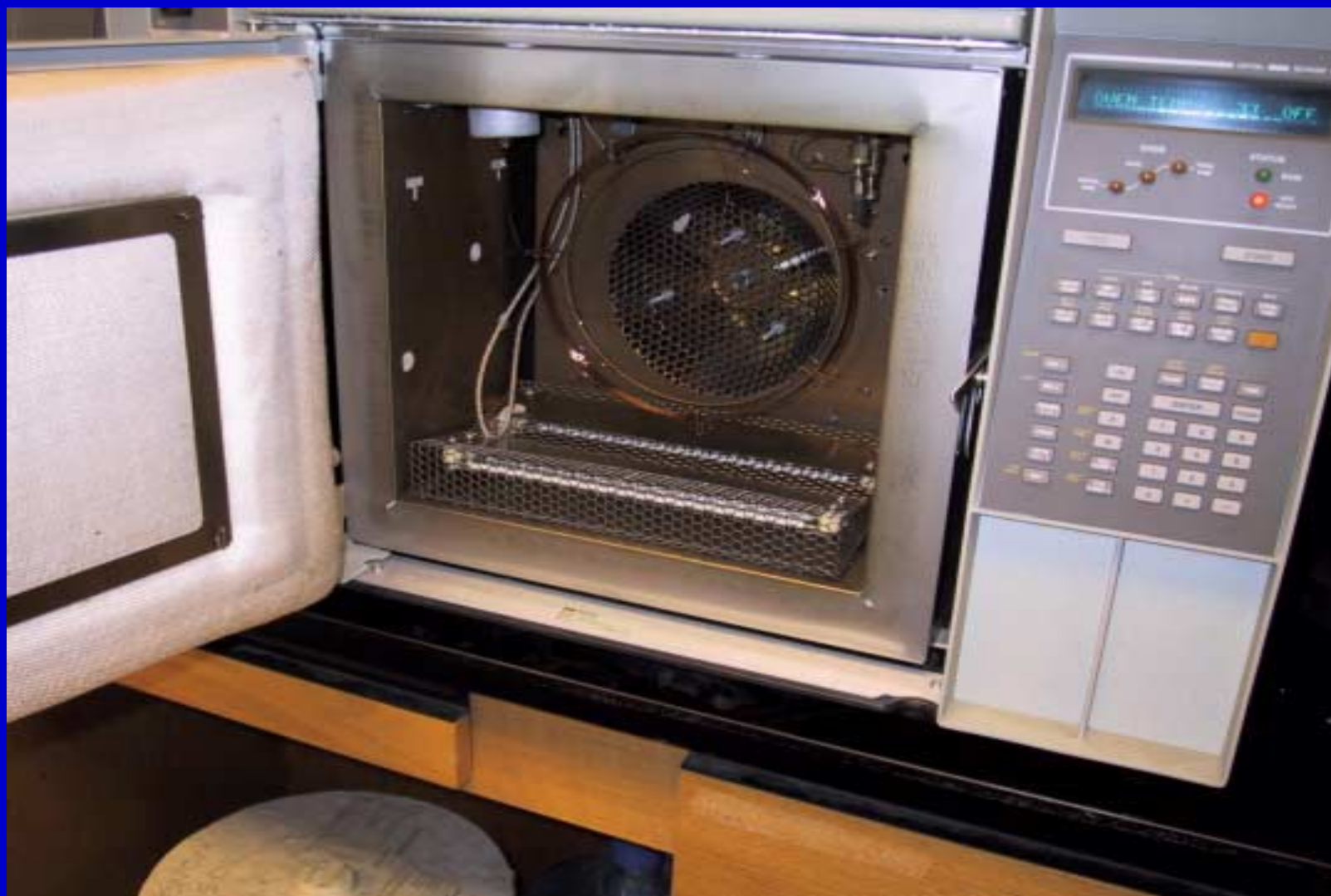
GC Racer Heater Installed in an Agilent 5890
