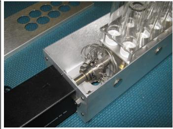
The septum of the vial is punctured by a 27 gage Luer-lok needle when the vial is inserted into the sampler.
