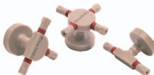
Quick mount tee, cross, and union, shown actual size (The red band protects the ferrule during assembly for shipment, and should be removed for actual makeup)
