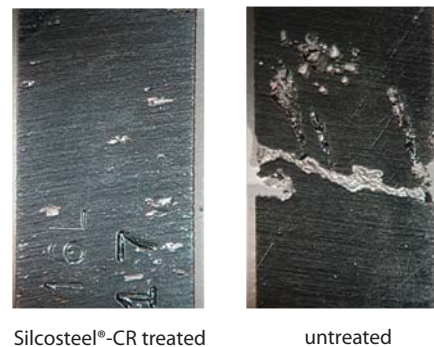
Figure 5 Silcosteel®-CR treated 316L stainless steel coupons show no crevice corrosion and only slight pitting corrosion after 72-hour exposure to ferric chloride; untreated coupons exhibit severe crevice corrosion.
