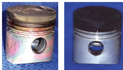
Figure 2 A Silcosteel®-AC-treated piston (left) shows dramatically less coke buildup than an untreated diesel piston (right). 2
