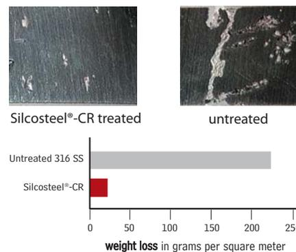
**Figure 3** Silcosteel®-CR treated stainless steel shows no sign of attack after 4000-hour salt spray exposure, per ASTM B117.
