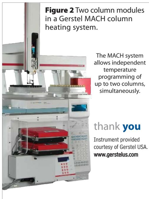
**Figure 2** Two column modules in a Gerstel MACH column heating system.
