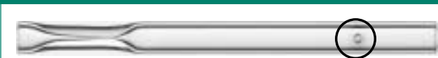
Figure 1—The drilled hole in a Uniliner® injection port liner makes direct injection possible with EPC systems by equalizing pressure in the injection port.
