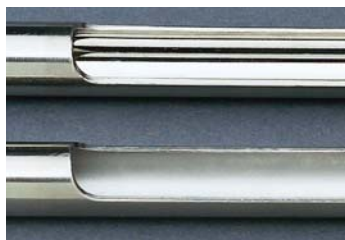
Top: electropolished finish, surface roughness average number: 5-10. Bottom: conventional finish, surface roughness average number: approx. 23-27.
