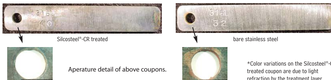
Figure 5 Silcosteel®-CR treated 316L stainless steel coupons show no corrosion as a result of salt spray testing; bare coupons show rusting at aperture.*
