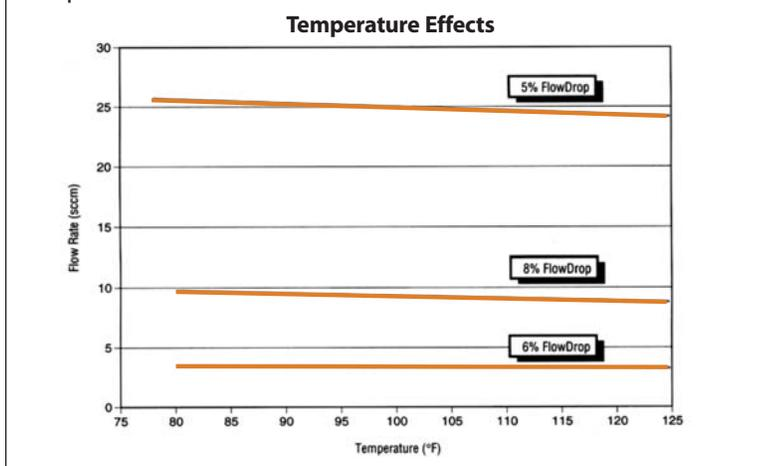
**Figure 5** A flow controller will maintain a constant sample flow until it is unable to maintain a stable pressure differential across the critical orifice.
