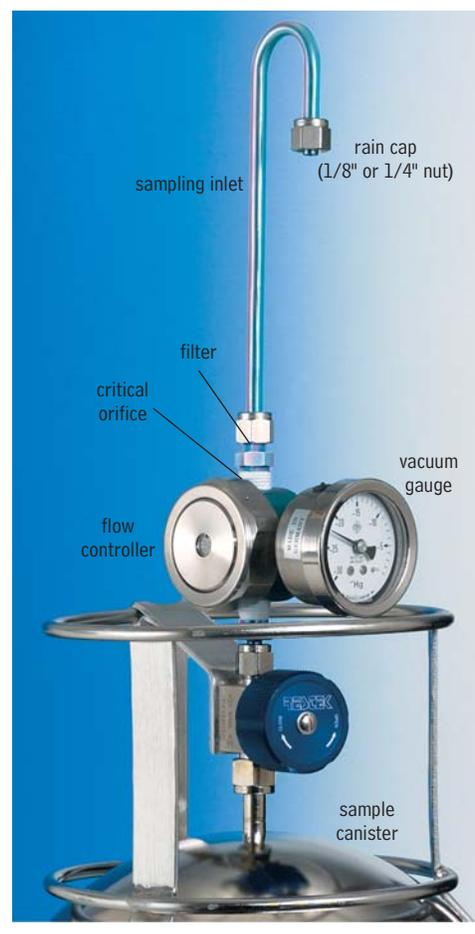
**Figure 2** Filters used in sampling trains.
