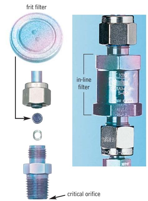
**Figure 3** Flow controller & critical orifice.
