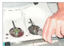
Use the larger end to tighten the split/splitless weldment nut.
