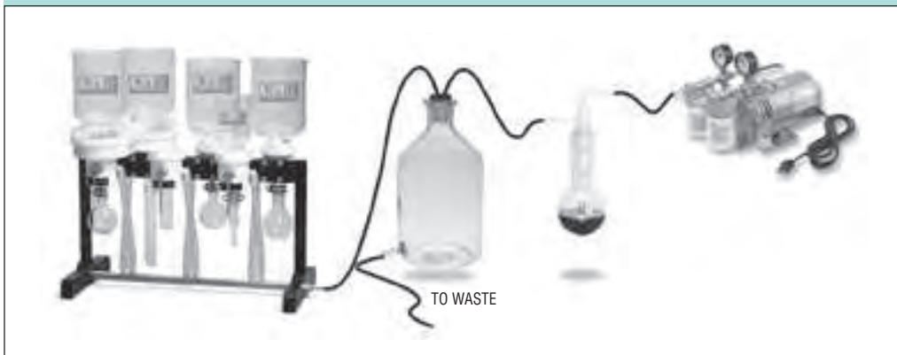
A Manifold B Tubing C Aspirator D Trap in Ice Bath E Vacuum Pump
