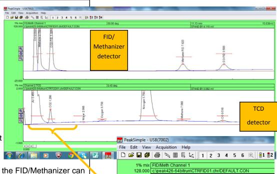
CO2 to methane so the FID/Methanizer can detect those molecules with the same sensitivity as methane and other hydrocarbons. The TCD responds to all molecules including water.
