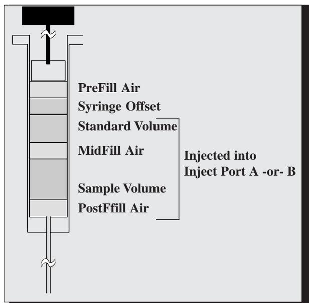
**Example 3 - Using Syringe Offset and Standard Offset**
