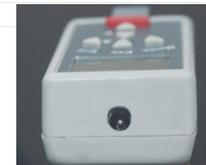
3. The pipette can be charged in both working and sleeping modes. The pipette can be used during charging also.
