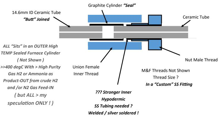
"H2 SITE" Ceramic Tube Graphite Seal Joiner
