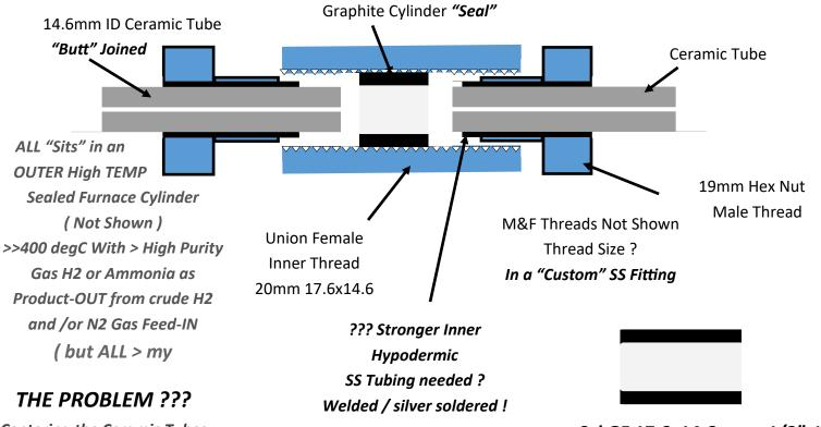
Centering the Ceramic Tubes whilst tightening
