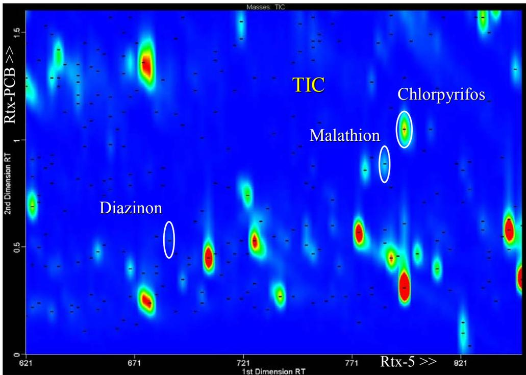
**Figure 3.** Contour plot of organophosphate pesticides in an ash leaves extract. Note how separations are occurring in two dimensions, and where Malathion and Chlorpyrifos have been separated in the second dimension from substantial matrix interferences (at a first dimension retention time of approximately 800 seconds).
