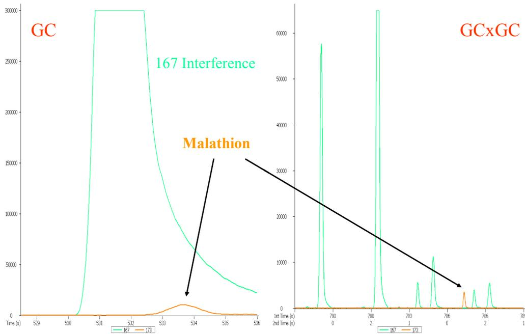
**Figure 6.** Linear chromatograms for one-dimensional (GC) and two-dimensional (GCxGC) analyses of Malathion in ash leaves. Malathion coelutes with a large matrix peak in GC, but is easily separated from this same compound using GCxGC.
