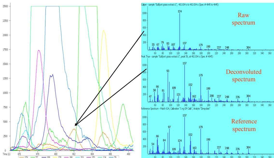
**Figure 1.** Chromatogram of 50 pg Diazinon (orange peak) in an ash leaves extract plotted with ions representing the matrix. The raw spectrum taken at the peak apex for Diazinon is representative of the matrix interferences. The deconvoluted TOF mass spectrum matches well with the reference spectrum.
