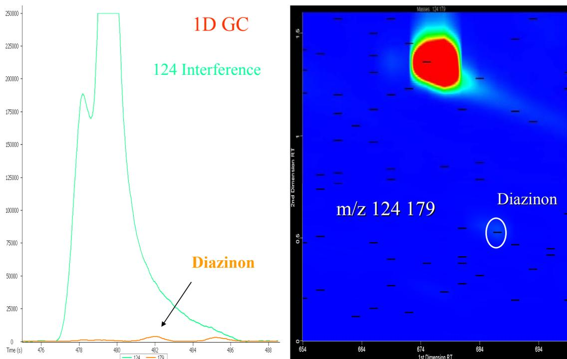
**Figure 7.** One-dimensional GC (1D GC) and GCxGC (contour plot on right) analyses for Diazinon in ash leaves. The matrix interference that contains substantial 124 ion and is coeluting with Diazinon in 1D GC is easily resolved from Diazinon using GCxGC. The peak containing the 124 ion is the large red spot in the contour plot.
