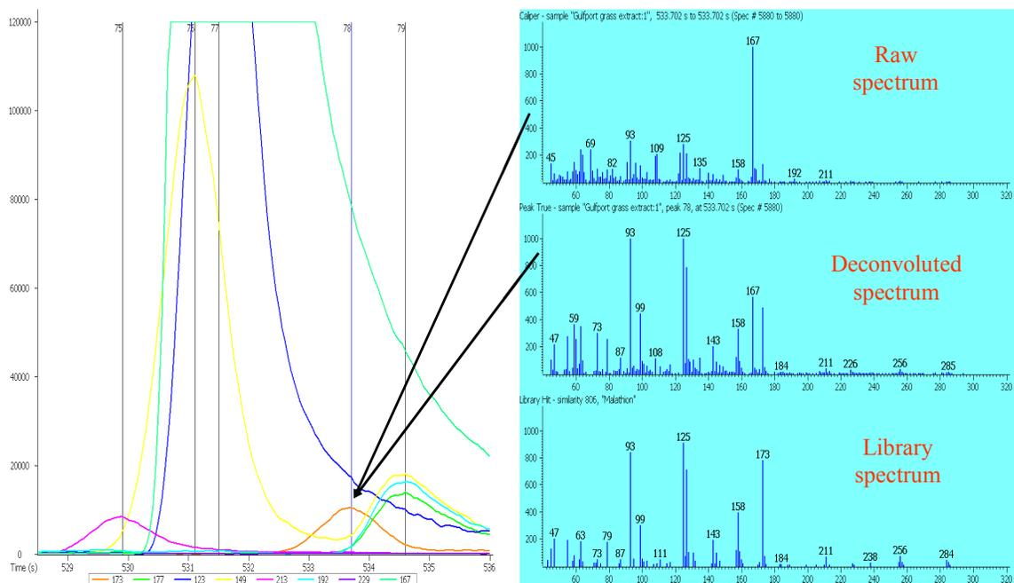
**Figure 2.** Chromatogram of 125 pg Malathion (orange peak) in an ash leaves extract plotted with ions representing the matrix. The raw spectrum taken at the peak apex for Malathion hardly hints that Malathion may be present. The deconvoluted TOF mass spectrum, even though it contains some residual 167 ion from the huge matrix interference, matches well with a library spectrum.
