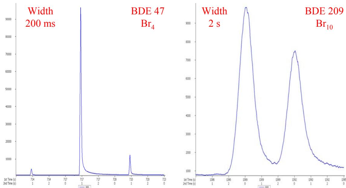
**Figure 5.** Linear chromatograms showing modulated peaks for BDEs 47 (tetrabromo) and 209 (decabromo). 50 spectra/second is an appropriate acquisition rate for the 200 ms wide peaks of BDE 47, but the rate is too fast for the broad peaks of BDE 209 (which results in a sensitivity decrease).
