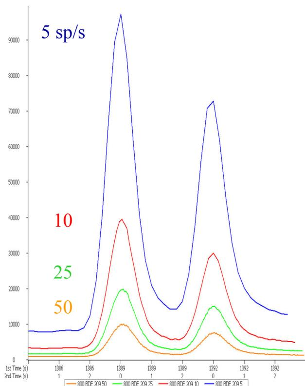
**Figure 7.** Linear chromatograms for modulated BDE 209 at original acquisition rate of 50 spectra/second (orange) and when sample reduction rates (of 2, 5, and 10) were used in the ChromaTOF Resample feature to produce new files at 25 (green), 10 (red), and 5 (blue) spectra/second. The enhanced peak responses are due to spectral summing.
