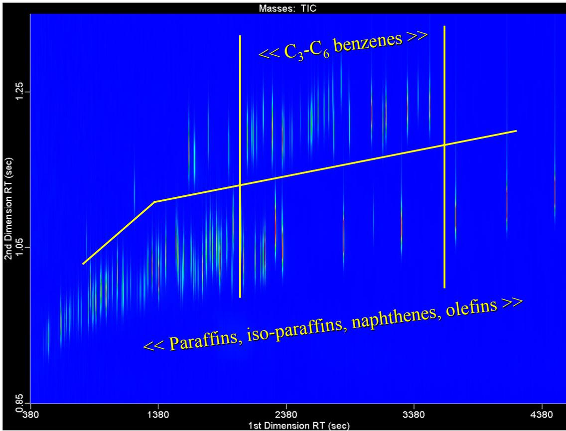
**Figure 1.** Contour plot of PIANO mix analyzed with GCxGC-TOFMS. The vertical yellow lines denote the first dimension retention area for processing the C<sub>3</sub>-C<sub>6</sub> benzenes. The horizontal yellow line is used only to mark the second dimension separation of aliphatics and aromatics.
