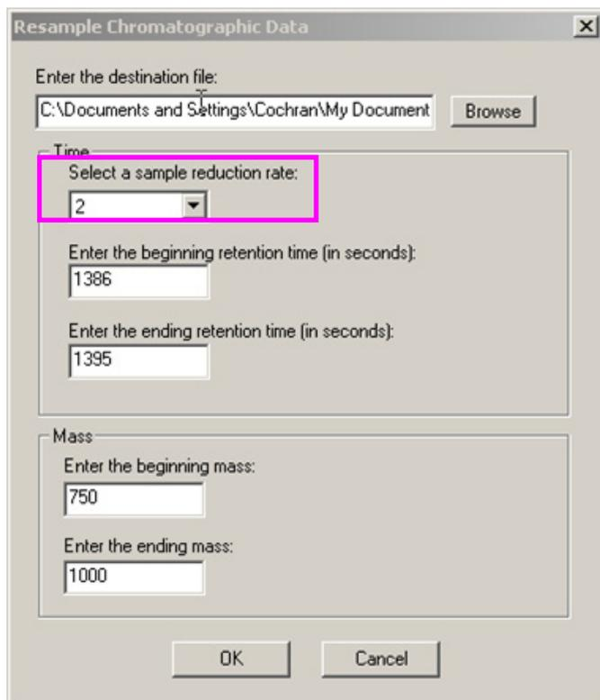
**Figure 6.** Dialog box showing Resample for BDE 209. Because the data acquisition rate was too fast for the broad peaks, a sample reduction rate of 2 was used for the retention time range for where BDE 209 eluted.
