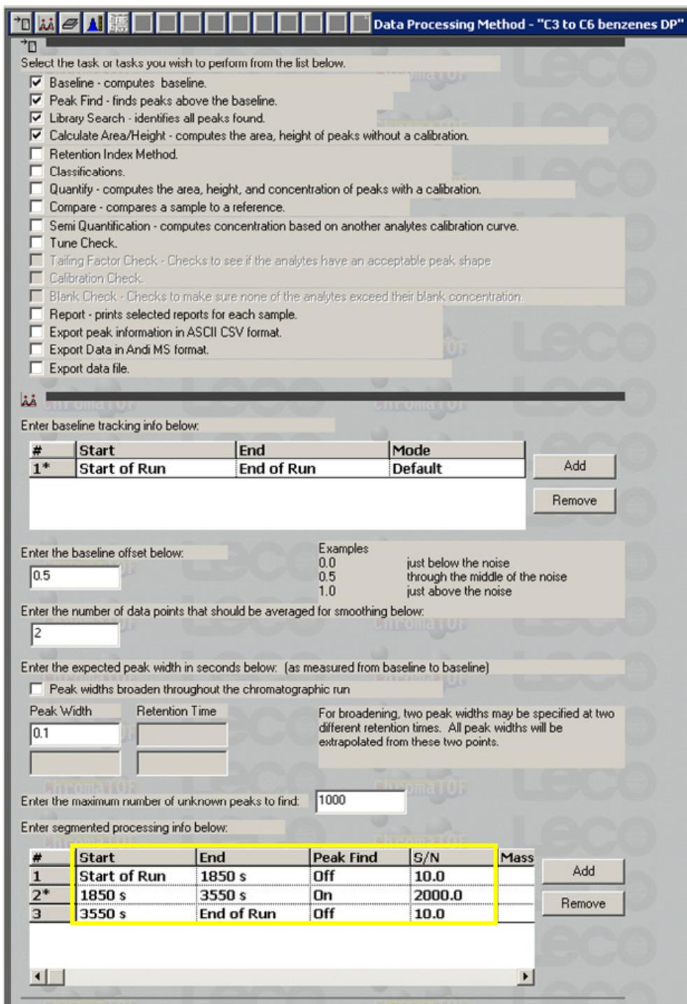
**Figure 2.** Segmented processing capability of ChromaTOF where peak finding can be restricted across a narrow retention time range.
