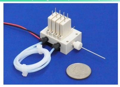
This module meters liquid for dispensing. Every time the button on the controller (external input also possible) is pushed, the module releases the liquid metered by the sample loop from the needle. Its small dimensions of  $38.3 \times 41.3 \times 37.4$ mm and light weight of approx. 25g enable it to be mounted on moving elements.
