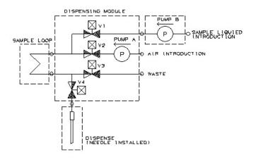
This is just an example of valve modules using our SMV series of shape memory alloy driven ultra-slim valves. The use of SMVs realises significant miniaturisation of various valve modules. In addition, prices are competitive, helping to reduce the cost of your modules.
