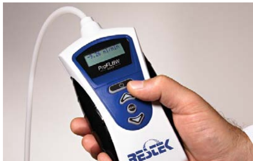
Figure 5 LED displays the measured flow value.
