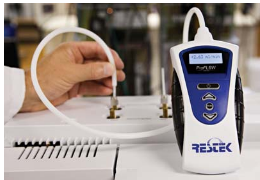
Figure 5 LED displays the measured flow value.
