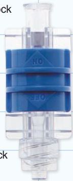
97337 Up To 1200psi Body: PC Slider: Acetal Collar: ABS Valve: Silicone
