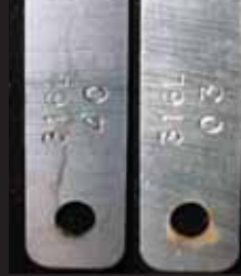
Silcosteel®-CR treated untreated
