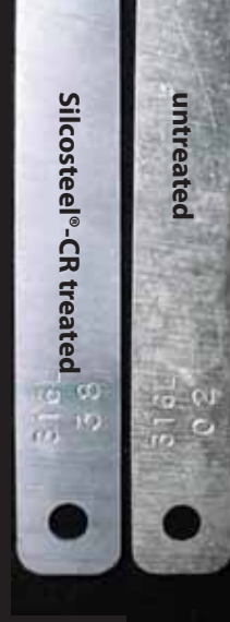
Silcosteel®-CR treated untreated
