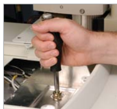
Turn counterclockwise to loosen jet.
