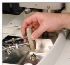
Remove FID cell assembly.
