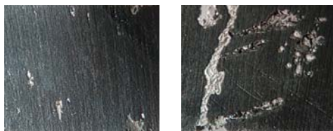
Figure 1 Silcosteel®-CR treated 316L stainless steel shows no crevice corrosion and only slight pitting corrosion, while bare 316L stainless steel exhibits severe crevice corrosion.
