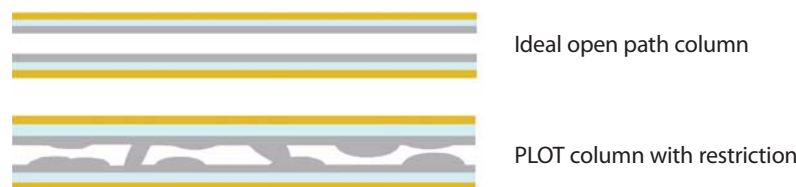
Figure 2 Inconsistent coating thicknesses result in restrictions that cause significant variation in flow.
