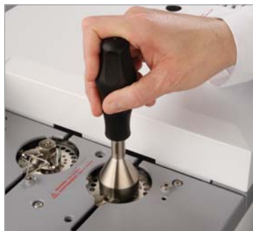
Simply slip the Weldment Removal Tool over the weldment, then twist and remove. For speed and efficiency, the weldment stays secured in the Weldment Removal Tool until you reattach it.
