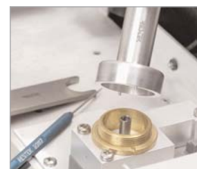
Easily loosens the nut by aligning the two pins on the bottom of the wrench with the two open slots on the nut...
